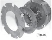
2a). Ensure the marked Hub drive tooth is engaged with the outlined drive slot(s) in the Carbon plates.
