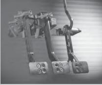
The bulkhead mounted type with master cylinders being located in the engine or front compartments. A lightweight aluminium base, and ergonomic steel and alloy pedals offer the user the ultimate control in this critical area. Uses conventional Master Cylinders e.g. CP2623.
