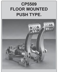
This is a general purpose floor mounted pedal box which utilises the latest high efficiency CP7854 push type master cylinders. Minimum hysteresis and balance variation are assured by the use of needle roller bearings in the centre trunnion and ball bearing pedal pivots.
