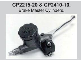
CP2410-10 - Bore Size 0.70". - Identified by two grooves <u>- Repair Kit CP2410-1RK</u> <u>- Lever CP2233-20</u> CP2215-20 - Bore Size 0.625" (5/8"). - Identified by single groove. <u>- Repair Kit CP2215-20RK</u> <u>- Lever CP2233-20</u>
