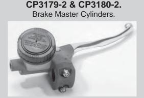
CP3179-2 - Bore Size 0.625" - Identified by single groove <u>- Repair Kit CP3179RK</u> <u>- Lever - CP2233-18</u> CP3180-2 - Bore Size 0.70". - Identified by two grooves. - Repair Kit CP3180RK - Lever - CP2233-18
