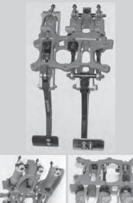
This unique pull type bulkhead mount design with master cylinders being located in the engine or front compartments allows the pushrod to remain in line eliminating all side loads making it one of the most efficient pedal box on the market. It's lightweight aluminium base, and ergonomic steel and alloy pedals offer the user the ultimate control in this critical area.
