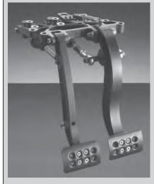
This multi ratio push type pedal box allows the pushrod to remain straight, eliminating all side loads therefore making it very efficient. The master cylinders connect directly to a high efficiency balance bar. 24.00
